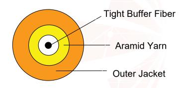
900µm tight buffer fiber,lszh, aramid yarn, flame-retardant jacket (UL-94 VO) Excellent stripping performance of tight buffer fiber Suited to SM fiber and MM fiber
